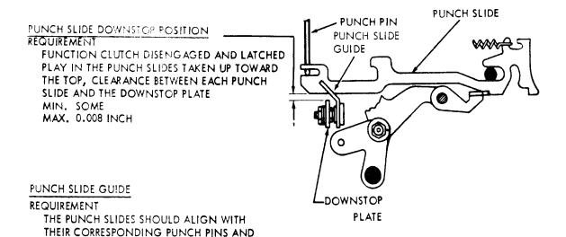
BE FREE OF BINDS AFTER TIGHTENING THE GUIDE MOUNTING STUDS. EACH PUNCH SLIDE SHOULD RETURN FREELY AFTER BEING PUSHED IN NOT MORE THAN 1/16 INCH.
